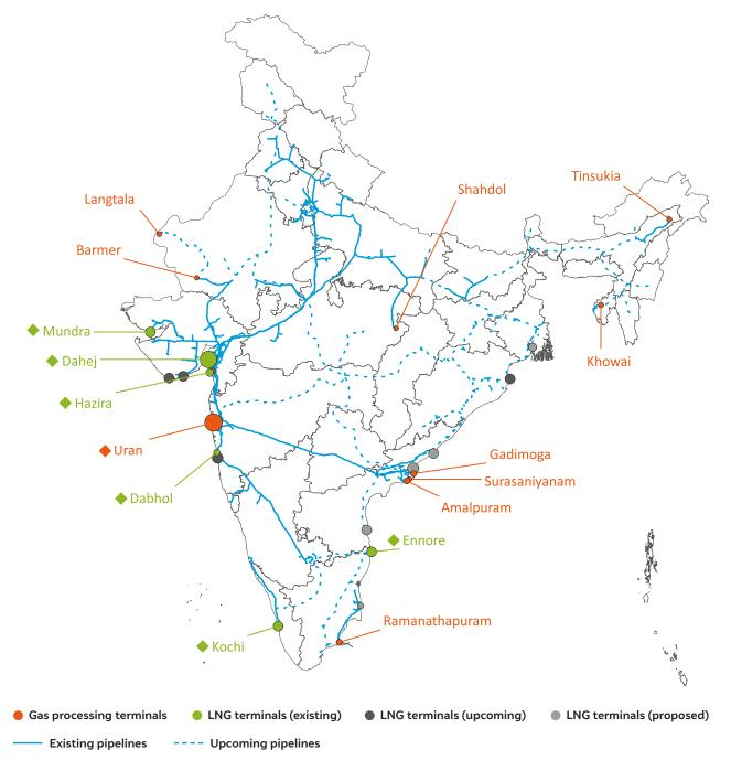
Figure 12 Possible injection point locations for blending hydrogen with piped natural gas
