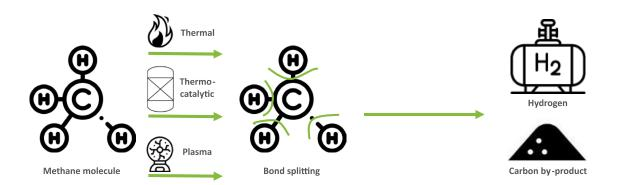
Figure 1 Natural gas (methane) pyrolysis produces solid carbon as a by-product with no greenhouse gas emissions
