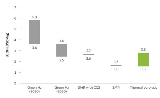
Figure 9 Hydrogen from natural gas pyrolysis is cheaper than the water electrolysis route and comparable with SMR with CCS
